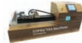
Material Testing: COPRA® FEA Bendtester
